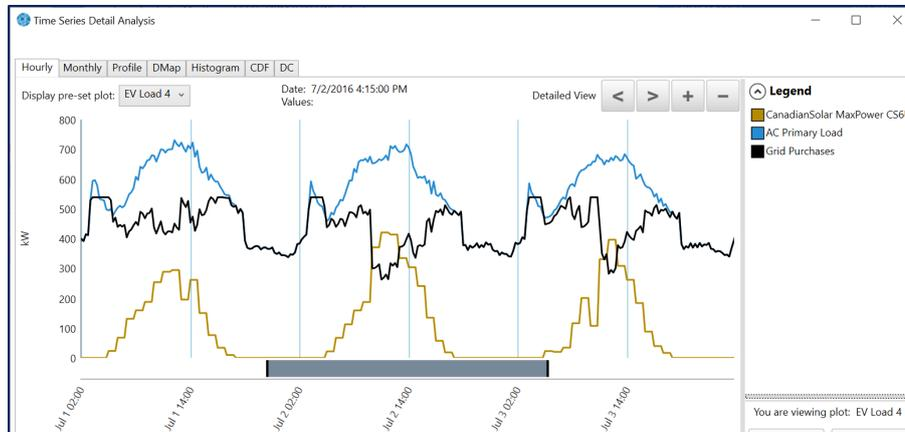
**Figure 6.1: Detailed view – total electrical load, solar production, energy storage charging/discharging.**
